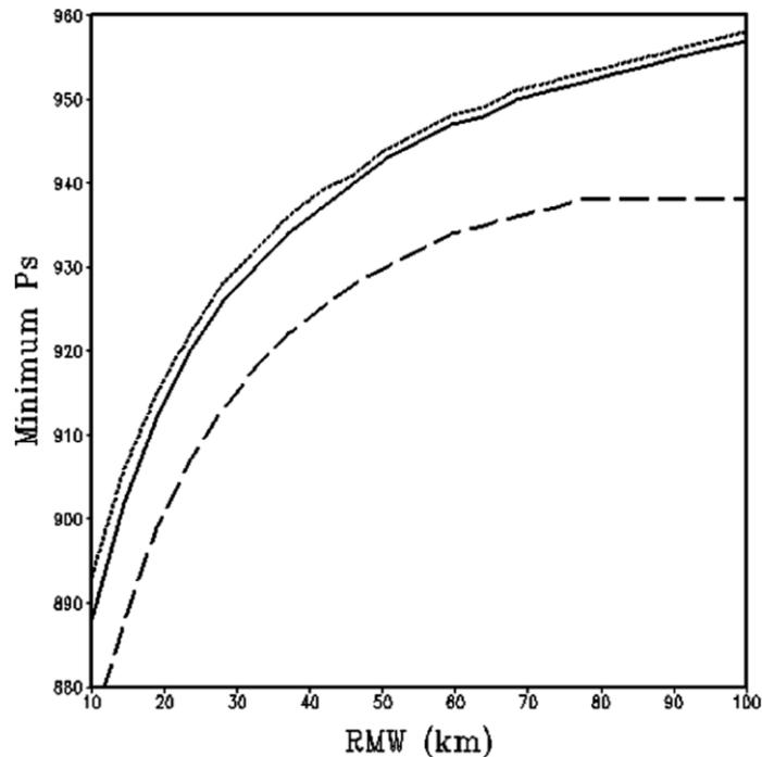
**Figure 3. Potential intensity as a function of RMW with different drag ( $C_d$ ) and heat exchange ( $C_h$ ) coefficients under high wind conditions ( $>35$  m/s). Solid: with constant  $C_d$  and  $C_h$  under high winds. Dotted: with  $C_d$  and  $C_h$  under high winds extrapolated based on the linear wind-exchange coefficient relations attained in low-to-moderate wind regimes. Dashed: different from the dotted with only  $C_d$  leveling off under high winds (from Shen 2006).**
